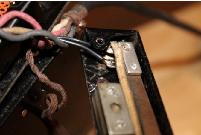
We need to connect some new wire to the soldering terminals on the receiver switch. These wires will eventually lead to the button terminals on the Bluetooth headset.
