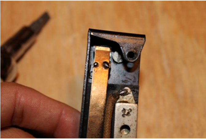
Top view of soldered switch plates.
